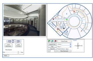
The VMAP software shows 360° recorded video on the left and a floor plan with calculated routes, recorded paths and items of interest shown on the right.
