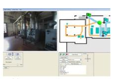
VMAP Nuclear can capture imagery of your plant's buildings and facilities that helps engineers, work planners, and maintenance workers see into the intricate facility without risking unnecessary worker exposure.
